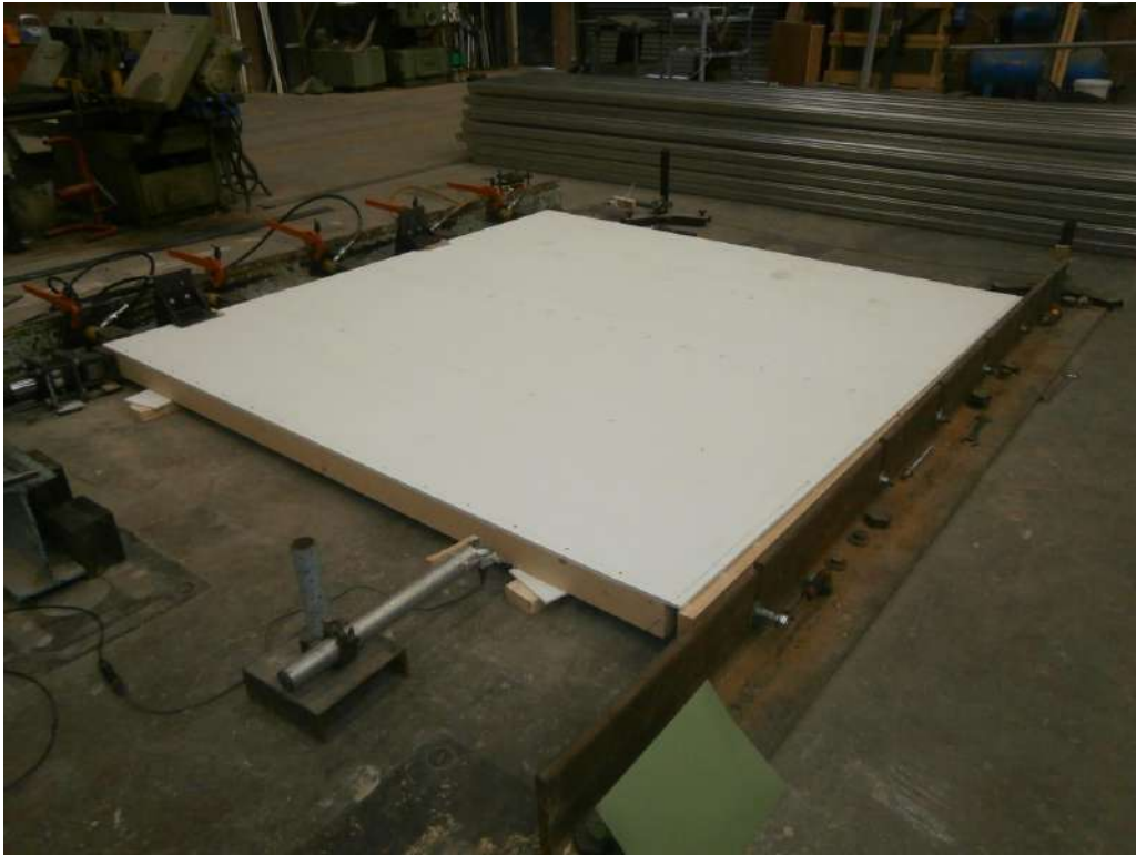
Plate 1 - General View of Racking Test Arrangement
