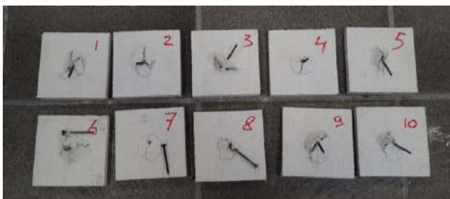
Photo 10 Failure mode 12 mm board.
