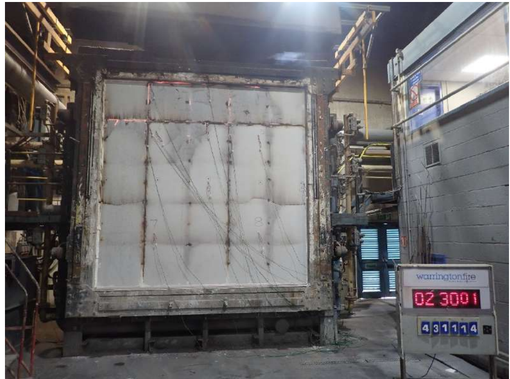
The unexposed face of the test specimen after 150 minutes of testing
