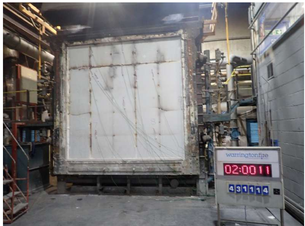
The unexposed face of the test specimen after 120 minutes of testing
