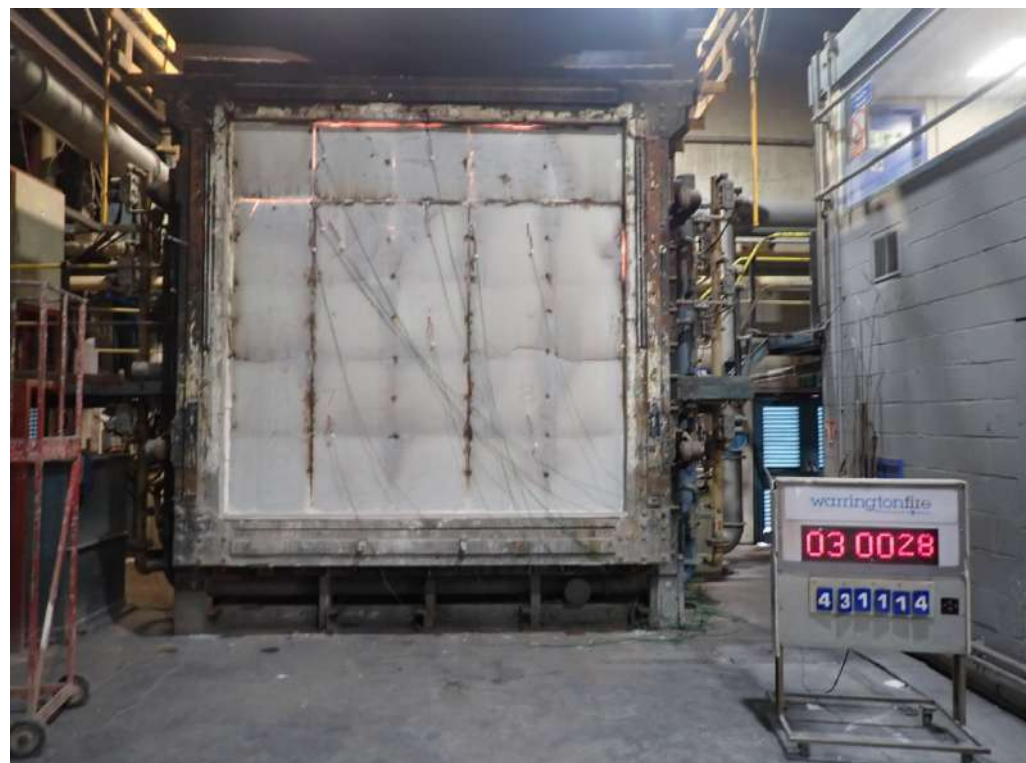
The unexposed face of the test specimen after 180 minutes of testing
