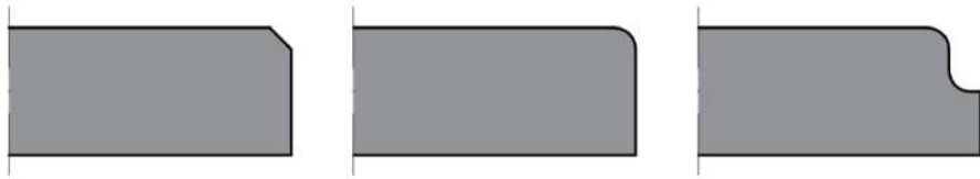
Figure 1.8 – Edge machining. Bevel, rounding and milling.
