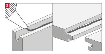
Apply EGGER Joint & Joist Adhesive directly to the groove and shoulder of the profile joint, continuing down the length of each board to ensure that the entire joint is bonded once the boards are butted tightly together. Adhesive should foam out of the board joint. This will enhance the protection of the joint. Excess adhesive should be left to dry.
