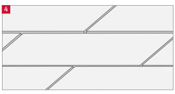
Apply EGGER Joint & Joist Adhesive along the next row of joists and stagger the next row of panels by approximately half a board to form a brick bond laying pattern. Repeat steps (excluding step 2) and note that care should be taken when walking on newly laid boards.
