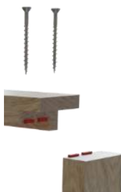
Trenched or Half Lapped Joint
