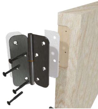
Example of hinge protection detail
