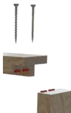
Trenched or Half Lapped Joint
