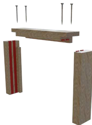
Trenched or Half Lapped Joint
