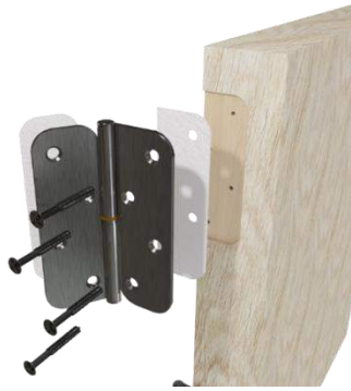
Example of hinge protection detail
