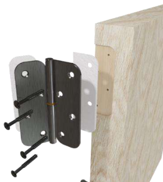
Example of hinge protection detail
