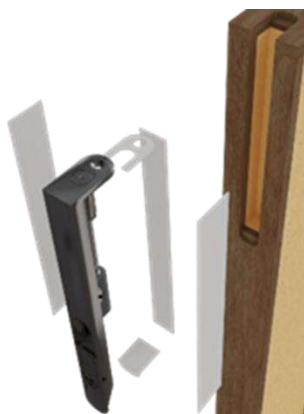
Flush bolt installation and intumescent protection
